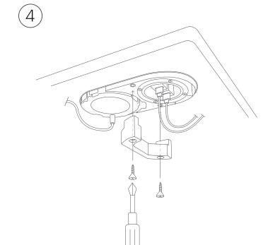
Use the two screws to fasten the bracket and secure the product.
