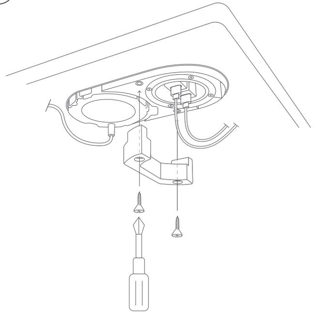
Use the two screws to fasten the bracket and secure the product.
