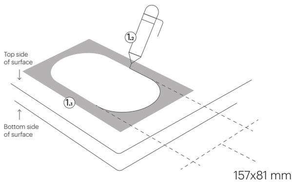
1.1 Position the mold on the top side of the surface.
